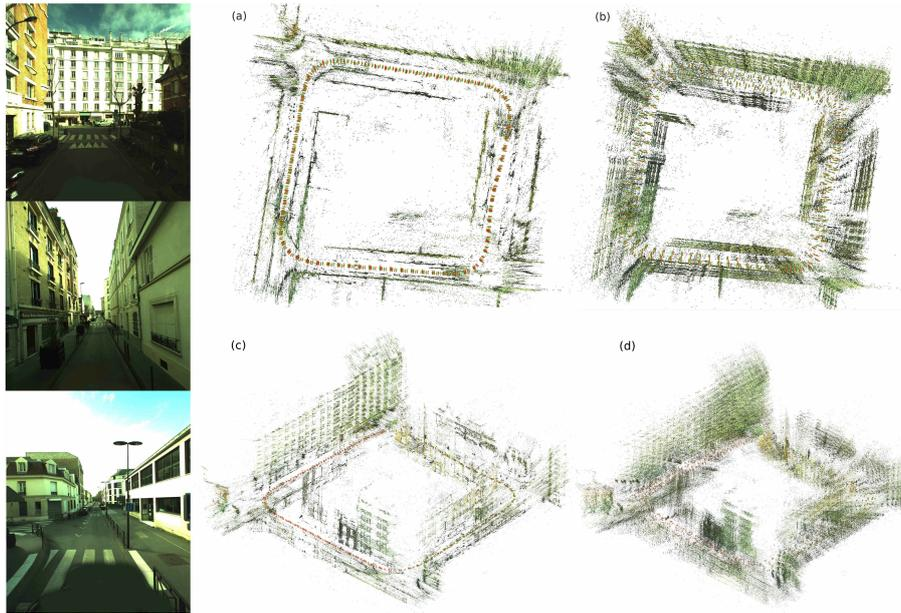
Figure 4. Left: excerpt from the CAR dataset. Right: (a) and (c) is the ground truth in top and side view; (b) and (d) is the equivalent  $E_{p+tri}$  result. Note the multiple facade effect in (b) and (d) due to error accumulation, and leads to a low frequency drift, as plotted in Figure 3.
