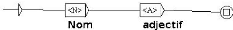
Figure 2: A simple finite state automaton that identifies sequences of nouns followed by adjectives in a text.
