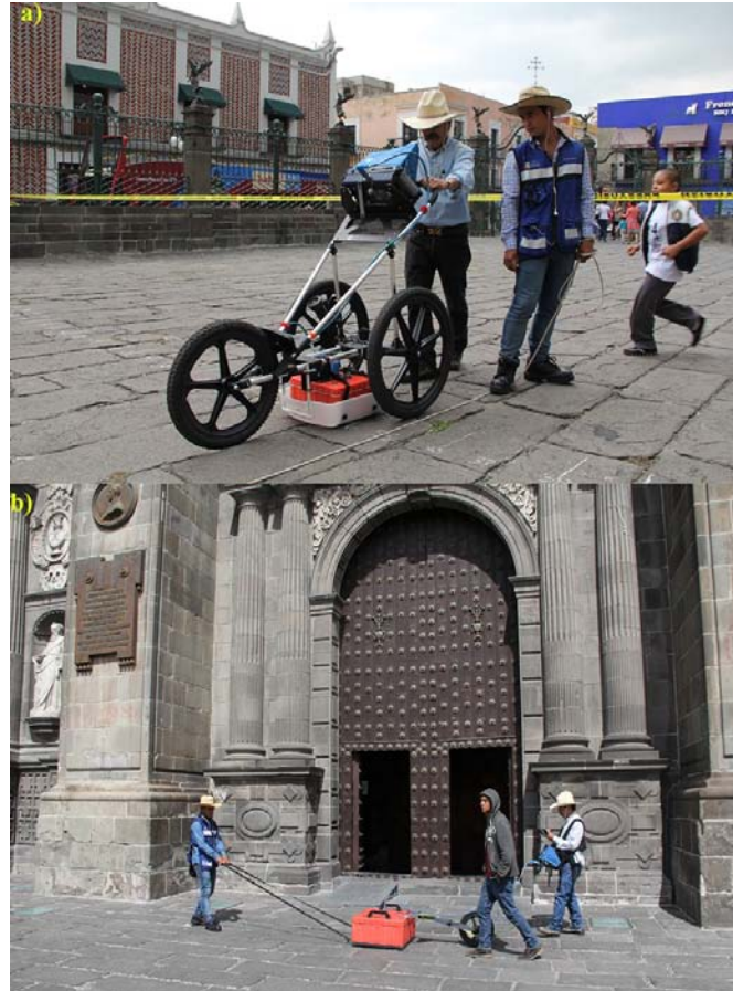
Fig. 2. GPR measurements in the atrium of Puebla Cathedral: a) With a 400 MHz frequency antenna. b) With a 200 MHz frequency antenna.
