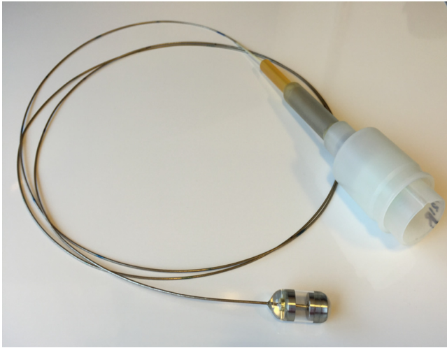
Fig. 1 TCE device comprising a capsule attached to the distal end of a flexible tether and terminated with an optical connector at the proximal end.
