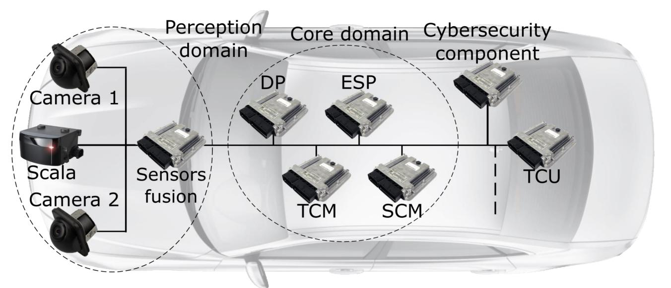
DP: Decisional Pilot TCM: Transmission Control Module ESP: Electronic Stability Program SCM: Steering Control Module TCU: Telematics and Communication Unit
