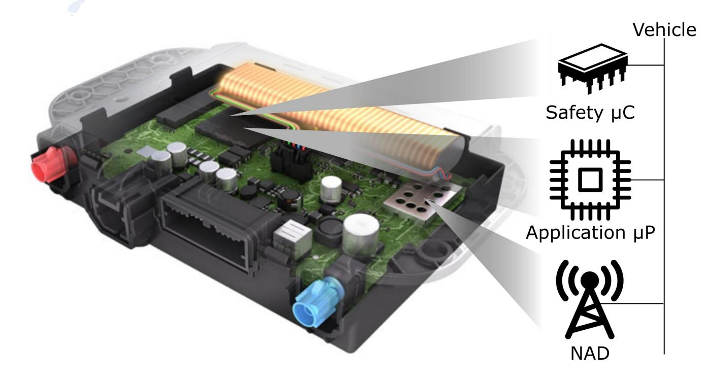
The following example is focused on a Telematics and Communication Unit (TCU), a privileged attack point. For the above TCU, two use cases are considered: a remote diagnostic (RD) and a remote control (RC).
