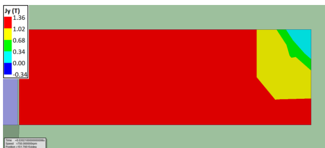
Fig. 15: Magnetisation map of a magnet in worst case during healthy mode 150°C and 40Nm.
