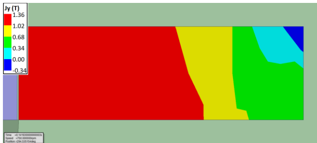
Fig. 16: Magnetisation map of a magnet in worst case during degraded mode for 150°C and 40Nm.
