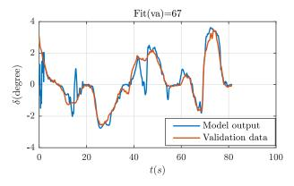
Fig. 10. Comparison of the TDNN model output  $\delta$  with the validation data (Rider 1, Input  $u_1$ , Output  $\delta$ )
