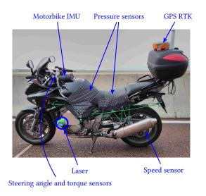
Fig. 2. The instrumented motorbike (VIROLO++ project)
