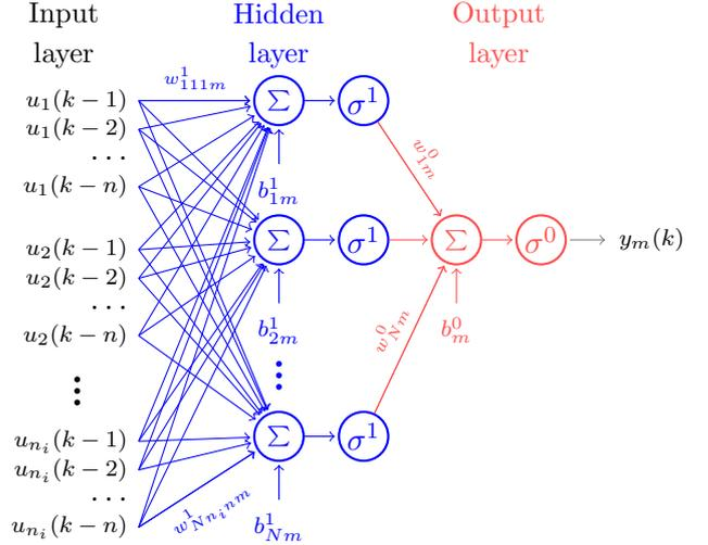
Fig. 9. MIMO TDNN with a single hidden layer
