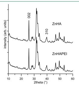
**Figure 1.** Powder X ray diffraction patterns of as prepared apatitic supports.
