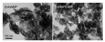
Figure 4. TEM images of the supports after (ZnHABP and ZnHAPEIBP) risedronate adsorption. Magnification in all TEM images is the same for direct comparison.
