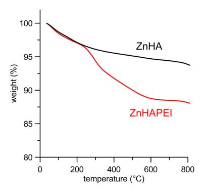
**Figure S1** – Thermogravimetric plot of ZnHA and ZnHAPEI. The weight loss centered at about 400°C is due to the combustion of organic fraction and allows to determine that ZnHAPEI sample contains about 5.9 wt% PEI.
