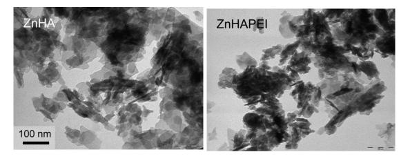
**Figure S2** – TEM images of the supports ZnHA and ZnHAPEI before risedronate adsorption. Magnification in all TEM images is the same for direct comparison.
