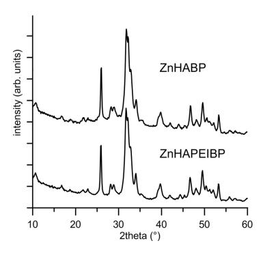
**Figure S4** – X-ray diffraction patterns of ZnHABP and ZnHAPEIBP. The adsorption of risedronate does not alter the crystallinity of pristine apatitic substrates and does not provoke precipitation of any other crystalline phase.
