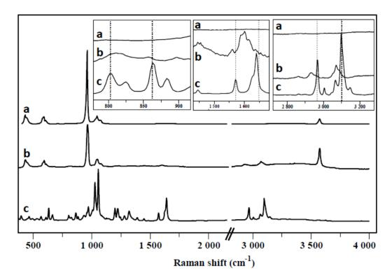
**Figure S5** – Raman spectra of ZnHA (a), ZnHABP (b), risedronate (BP) sodium salt (c). The insets focus each on a spectral domain (775-925 cm<sup>-1</sup>, 1375-1675 cm<sup>-1</sup> and 2700-3300 cm<sup>-1</sup>) to show the main characteristic vibration bands of risedronate molecule (pyridine ring, phosphonate group, C-H, C=C and C=N groups).
