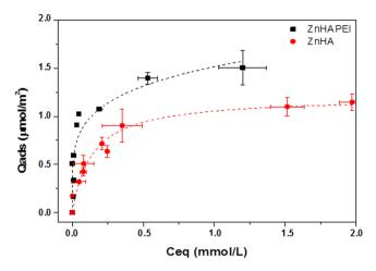
**Figure 2.** Adsorption isotherms of risedronate on Zn substituted hydroxyapatite (ZnHA) and PEI modified Zn substituted hydrox yapatite (ZnHAPEI) at pH 7.4 and 37 °C. The ZnHA and ZnHAPEI data are fitted with a Langmuir and a Freundlich isotherm, respectively.
