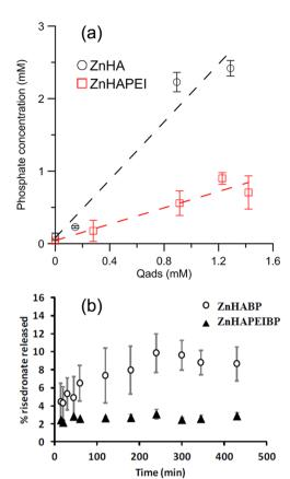
**Figure 3.** (a) Concentration of phosphate ions released in solution after BP adsorption as a function of the concentration of risedronate adsorbed on the powders, ZnHA and ZnHAPEI (1 mM KCl aqueous solution at pH 7.4 and 37  $^{\circ}$ C). (b) Risedronate released (wt %) from ZnHABP and ZnHAPEIBP supports as a function of time.
