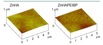
**Figure 5.** Atomic force microscopy images of the surfaces of disk shaped samples obtained by pressing as prepared ZnHA and ZnHAPEIBP powders into cylindrical molds and used for cell tests.
