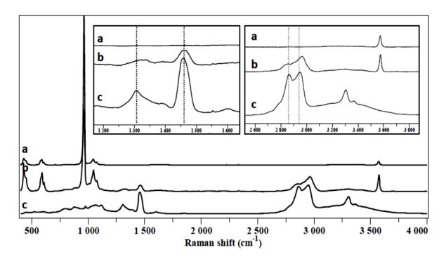
**Figure S3** – Raman spectra of ZnHA (a), ZnHAPEI (b), PEI (c). The two insets focus on two spectral domains (1150-1650 cm<sup>-1</sup> and 2550-3850 cm<sup>-1</sup>) showing especially the main characteristic vibration bands for CH and CH<sub>2</sub> groups in PEI molecule.
