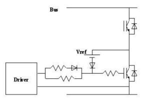
Fig. 5. clamping with ideal voltage source
