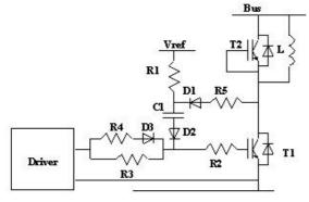
Fig. 6. Clamping circuit using a capacitor
