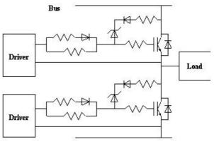
Fig. 3. Classical clamping (only one Transil diode shown for clarity)
