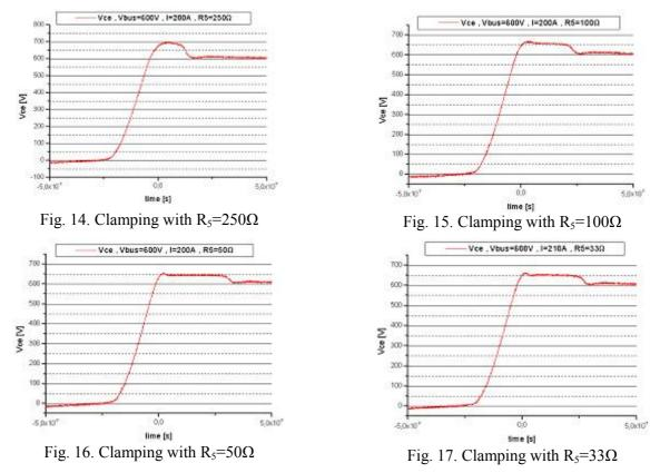
It can be noticed that the value of the over-voltage of  $V_{ce}$  is dependent on  $R_5$ . For low values of  $R_5$  (from 50 $\Omega$  to 33 $\Omega$ ), the over voltage is equal to 650V and is not reduced further. Much lower values will produce unwanted oscillations.
