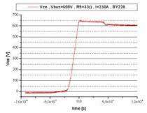
Fig. 10. Clamping with BY228 diode (D<sub>2</sub>)
