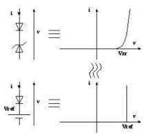
Fig. 4. Equivalence between transil diode and voltage source
