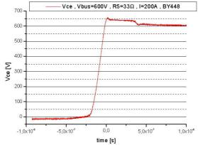
Fig. 11. Clamping with BY448 diode (D<sub>2</sub>)
