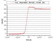
Fig. 9. Clamping with SiC diode (D<sub>2</sub>)
