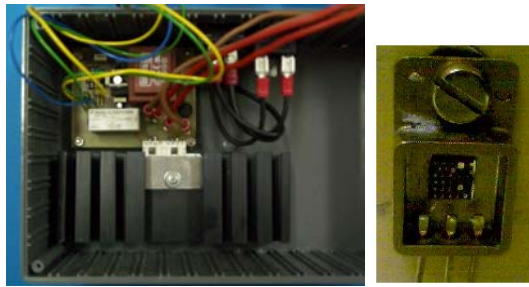
Fig. 14.- Short-circuit test set-up and encapsulated VJFET, on alumina (left) and metallic TO220 (right).
