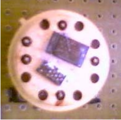
Fig. 10.- Packaged SiC ACCUMOS limiting device.
