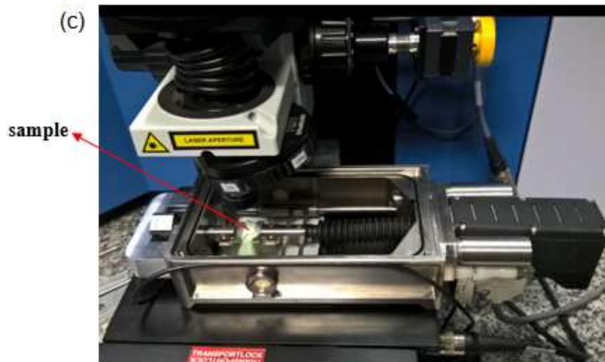
Figure 1- TMJ disc sample extracted from pig cadaver (the region of interest is highlighted) (a); photography of the hydro-chemo-mechanical device in a vertical set (b), and the photograph of the device coupled to a confocal Raman microscope (c).
