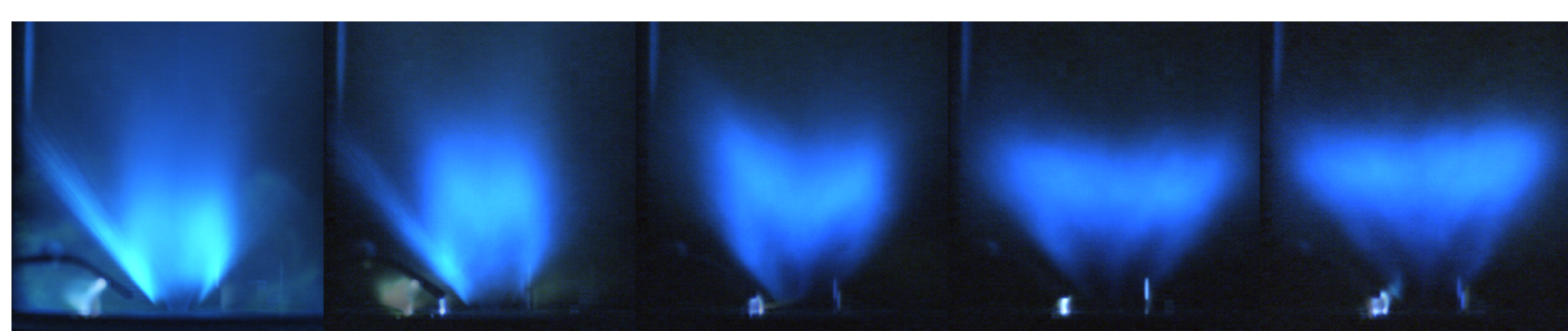
(a) 4.17 ms (b) 12.5 ms (c) 20.8 ms (d) 29.2 ms (e) 37.5 ms Experimental ignition sequence recorded by a high-speed camera with OH* filter [1].
