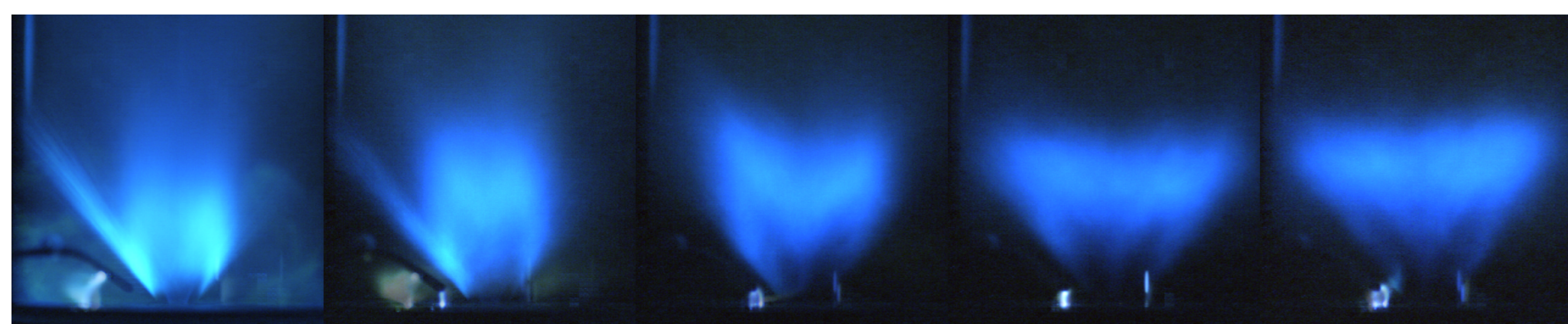
(a) 4.17 ms (b) 12.5 ms (c) 20.8 ms (d) 29.2 ms (e) 37.5 ms Experimental ignition sequence recorded by a high-speed camera with OH* filter [1].
