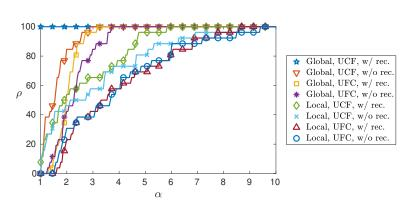
FIG. 5.3. Performance profile of the eight possible strategies to solve a BLR linear system over 26 real-life matrices.  $\rho$  (y-axis) indicates the percentage of matrices for which a given strategy requires less than  $\alpha$  (x-axis) times the flops required by the best strategy. For any given matrix, all eight strategies achieve roughly the same backward error.
