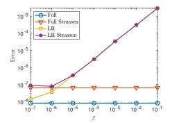
(B) Forward error (3.9) with multiplications performed in single precision, either classically or by Strassen's algorithm.
