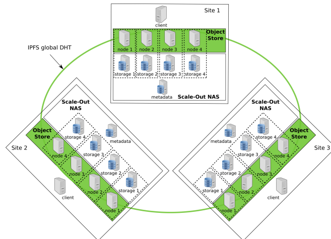
Figure 8. The Fog software architecture combining an object store (IPFS) and a Scale-Out NAS (like RozoFS).
