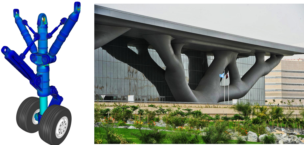
FIGURE 1. (Left) Shape and topology optimization of a landing gear by an industrial software (courtesy of ansys ) (right) The Qatar National Convention Center (architect: Arata Isozaki) has the typical outline of a topology optimized structure (licence Creative Commons)
