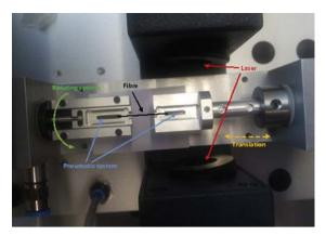
Fig. 3. Fibre dimensional analysis system.
