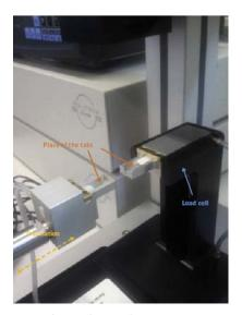
Fig. 4. Fibre tensile test system.
