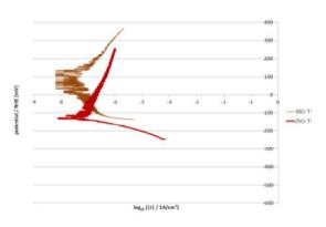
Figure 9: Tafel plots for the two Cr-richest alloys (Co-25 and 30 wt.%Cr)
