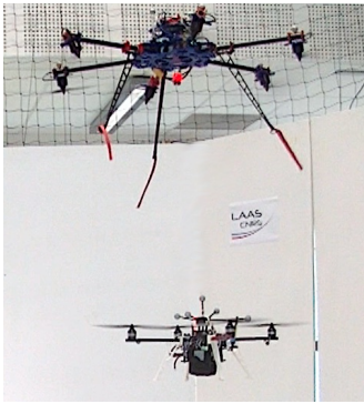
Fig. 4: The quadrotor flying stably beneath a 2.5 [Kg] hexarotor.
