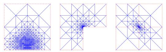
Figure 5: Graded meshes obtained by the newest-vertex bisection algorithm. Left: Peak problem, J = 10, and p = 3. Center: L-shape problem, J = 10, and p = 3. Right: Checkerboard O(10<sup>6</sup>), J = 10, and p = 3. The regions where the diffusion coefficient is constant are bordered by dashed lines.
