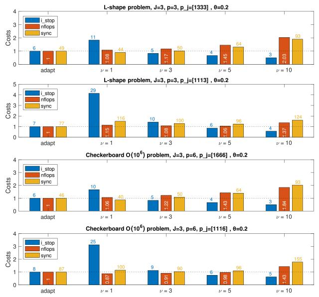
Figure 7: Comparison between a fixed number of (block-Jacobi) smoothing steps  $\nu$  on all levels (Definition 4.1 and its obvious modification for  $\nu \geq 1$ ) and the adaptive number of smoothing steps of Definition 7.1. Number of iterations  $i_s$ , floating point operations given by (8.1) relative with respect to Definition 7.1, and the number of global synchronizations by (9.6).
