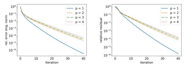
Figure 9: Nested cubes case: decay of the relative algebraic error (left) and the relative residual (right) for the hierarchy with  $p_j = 1$ ,  $j \in \{1, ..., J-1\}$ , J = 4. The solver of Definition 4.1 is stopped at iteration i = 40. nDoFs: 7 281 for p = 1, 55 649 for p = 2, 185 041 for p = 3, 435 393 for p = 4.
