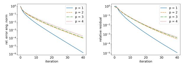
Figure 10: Checkers cubes: decay of the relative algebraic error (left) and the relative residual (right) for the hierarchy with  $p_j = 1$ ,  $j \in \{1, ..., J-1\}$ , J = 4. The solver of Definition 4.1 is stopped at iteration i = 40. nDoFs: 5 425 for p = 1, 40 033 for p = 2, 131 473 for p = 3, 307 393 for p = 4.
