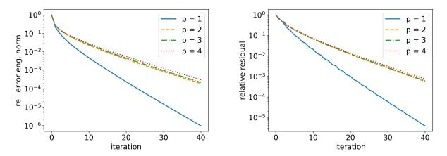
Figure 8: Cube case: decay of the relative algebraic error (left) and the relative residual (right) for the hierarchy with  $p_j = 1$ ,  $j \in \{1, ..., J-1\}$ , J = 4. The solver of Definition 4.1 is stopped at iteration i = 40. nDoFs: 5 501 for p = 1, 41 337 for p = 2, 136 693 for p = 3, 320 753 for p = 4.
