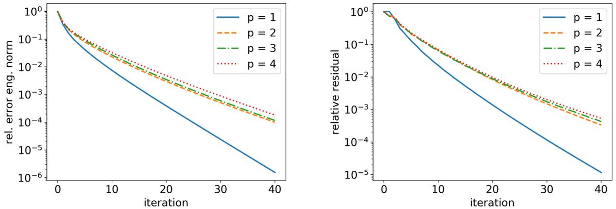
Figure 10: Checkers cubes: decay of the relative algebraic error (left) and the relative residual (right) for the hierarchy with  $p_j = 1, j \in \{1, \dots, J-1\}, J = 4$ . The solver of Definition 4.1 is stopped at iteration  $i = 40$ . nDoFs: 5 425 for  $p = 1$ , 40 033 for  $p = 2$ , 131 473 for  $p = 3$ , 307 393 for  $p = 4$ .
