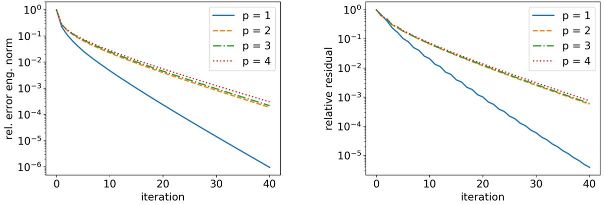
Figure 8: Cube case: decay of the relative algebraic error (left) and the relative residual (right) for the hierarchy with  $p_j = 1, j \in \{1, \dots, J-1\}, J = 4$ . The solver of Definition 4.1 is stopped at iteration  $i = 40$ . nDoFs: 5 501 for  $p = 1$ , 41 337 for  $p = 2$ , 136 693 for  $p = 3$ , 320 753 for  $p = 4$ .
