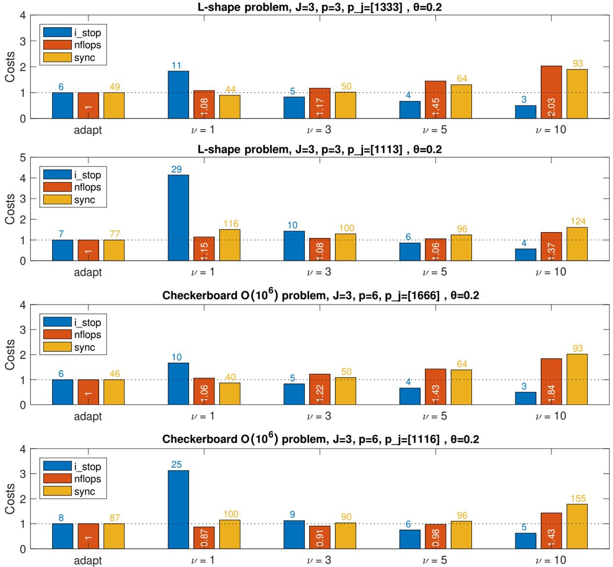
Figure 7: Comparison between a fixed number of (block-Jacobi) smoothing steps  $\nu$  on all levels (Definition 4.1 and its obvious modification for  $\nu \geq 1$ ) and the adaptive number of smoothing steps of Definition 7.1. Number of iterations  $i_s$ , floating point operations given by (8.1) relative with respect to Definition 7.1, and the number of global synchronizations by (9.6).
