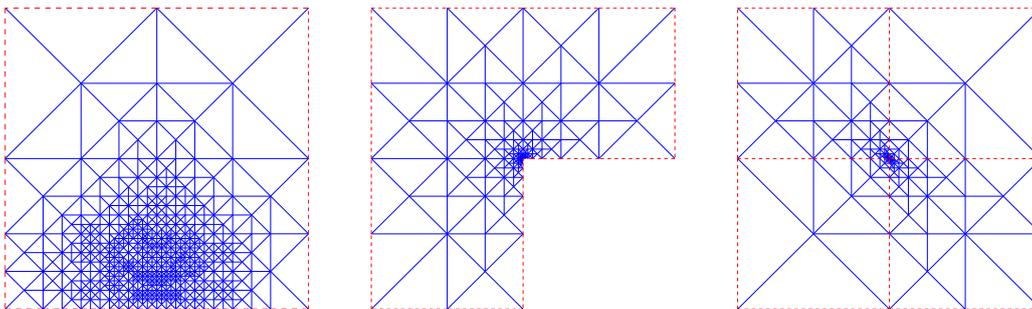
Figure 5: Graded meshes obtained by the newest-vertex bisection algorithm. Left: Peak problem,  $J = 10$ , and  $p = 3$ . Center: L-shape problem,  $J = 10$ , and  $p = 3$ . Right: Checkerboard  $O(10^6)$ ,  $J = 10$ , and  $p = 3$ . The regions where the diffusion coefficient is constant are bordered by dashed lines.
