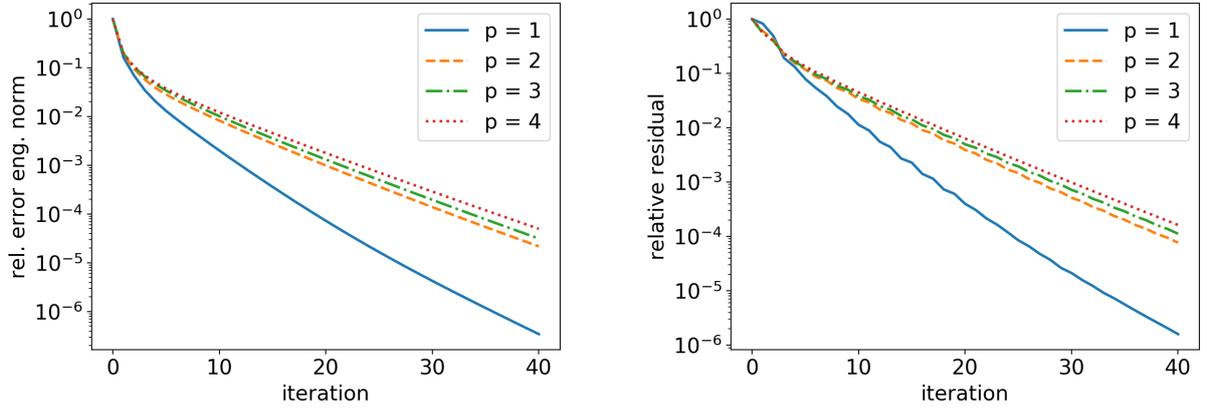
Figure 9: Nested cubes case: decay of the relative algebraic error (left) and the relative residual (right) for the hierarchy with  $p_j = 1, j \in \{1, \dots, J-1\}, J = 4$ . The solver of Definition 4.1 is stopped at iteration  $i = 40$ . nDoFs: 7 281 for  $p = 1$ , 55 649 for  $p = 2$ , 185 041 for  $p = 3$ , 435 393 for  $p = 4$ .
