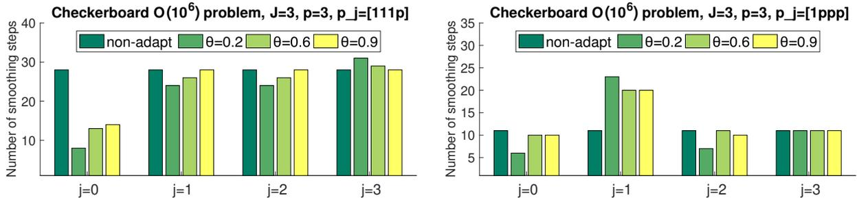
Figure 6: Number of smoothing steps per level for the Checkerboard case, polynomial degree  $p = 3$ , number of mesh levels  $J = 3$ , diffusion coefficient jump  $\mathcal{J}(\mathcal{K}) = O(10^6)$ , and mesh hierarchies with  $p_j = 1$  and  $p_j = p$ ,  $j \in \{1, \dots, J - 1\}$ .
