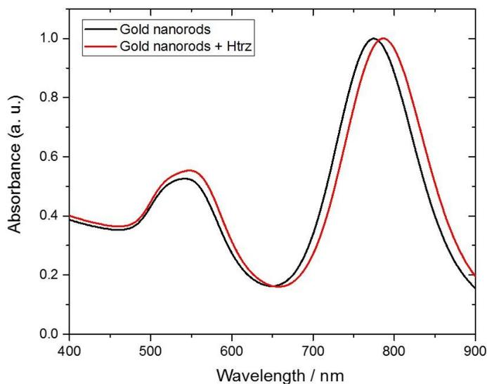
**Figure 1:** Absorption spectra of gold nanorods dispersion in water, stabilized by 5 mM of CTAB, before (black curve) and after addition of 1.8 M of Htrz ligand aqueous solution. (Nota: the concentration of 1.8 M is further used for the synthesis of the nanocomposites).
