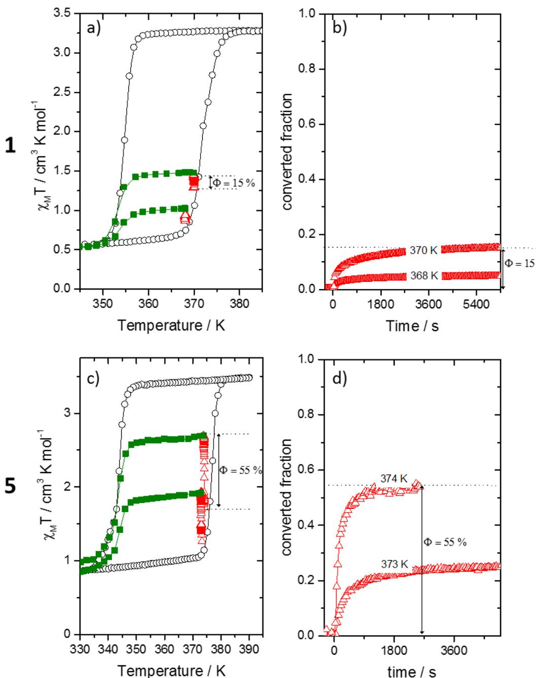
**Figure 6:** Photoswitching experiments performed on compounds **1** (top) and **5** (bottom), using a laser fluence of 15 mW/cm<sup>2</sup> centred at 830 nm. a) and c) report the hysteresis curve (o), the isothermal irradiations (Δ) and the following cooling curves (■). b) and d) report the converted HS fraction as function of time at two different temperatures.
