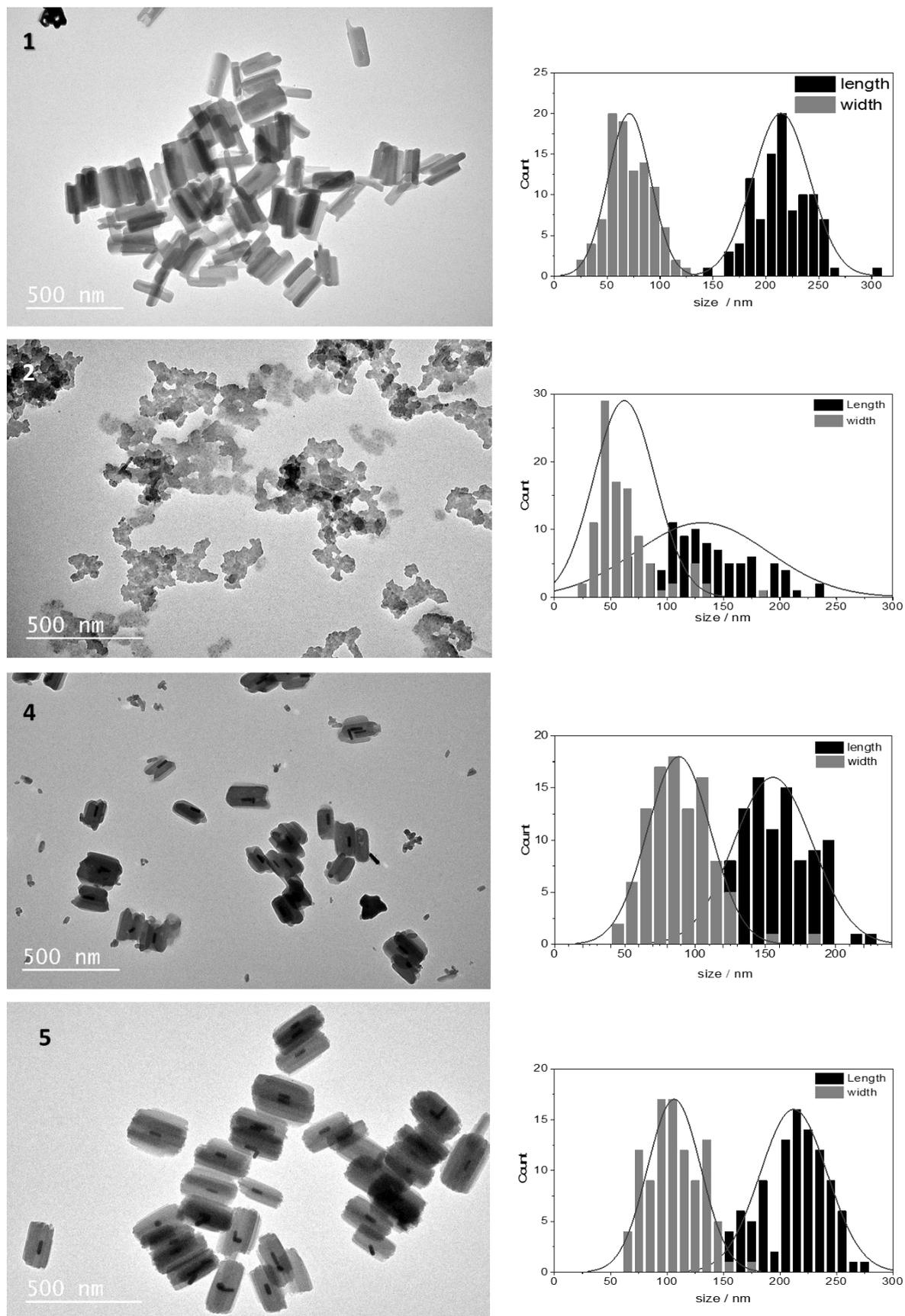
**Figure 2:** TEM images and size distributions of samples **1** ( $[\text{Fe}(\text{Htrz})_2(\text{trz})](\text{BF}_4)$ ) obtained from micellar synthesis), **2** ( $[\text{Fe}(\text{Htrz})_2(\text{trz})](\text{BF}_4)$ ) obtained from direct synthesis) and **4** and **5** ( $\text{Au}@[\text{Fe}(\text{Htrz})_2(\text{trz})](\text{BF}_4)$ ).
