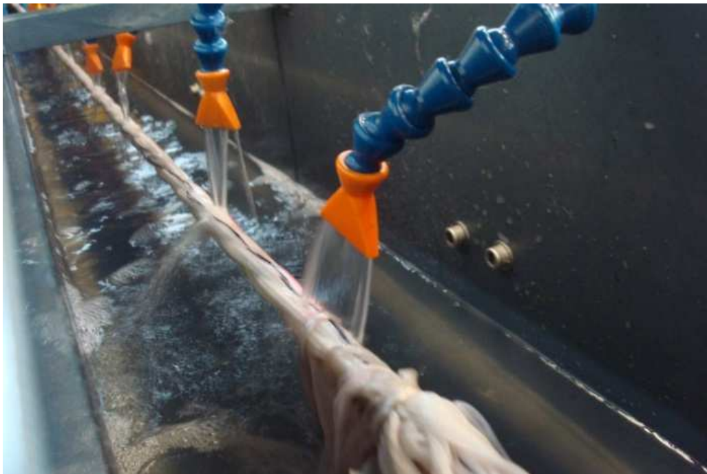
Figure. 2. Rope during a fatigue test
