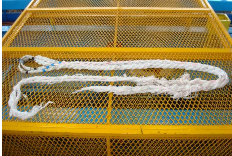
Figure 8. Failed sample after test, showing two broken parts superposed.
