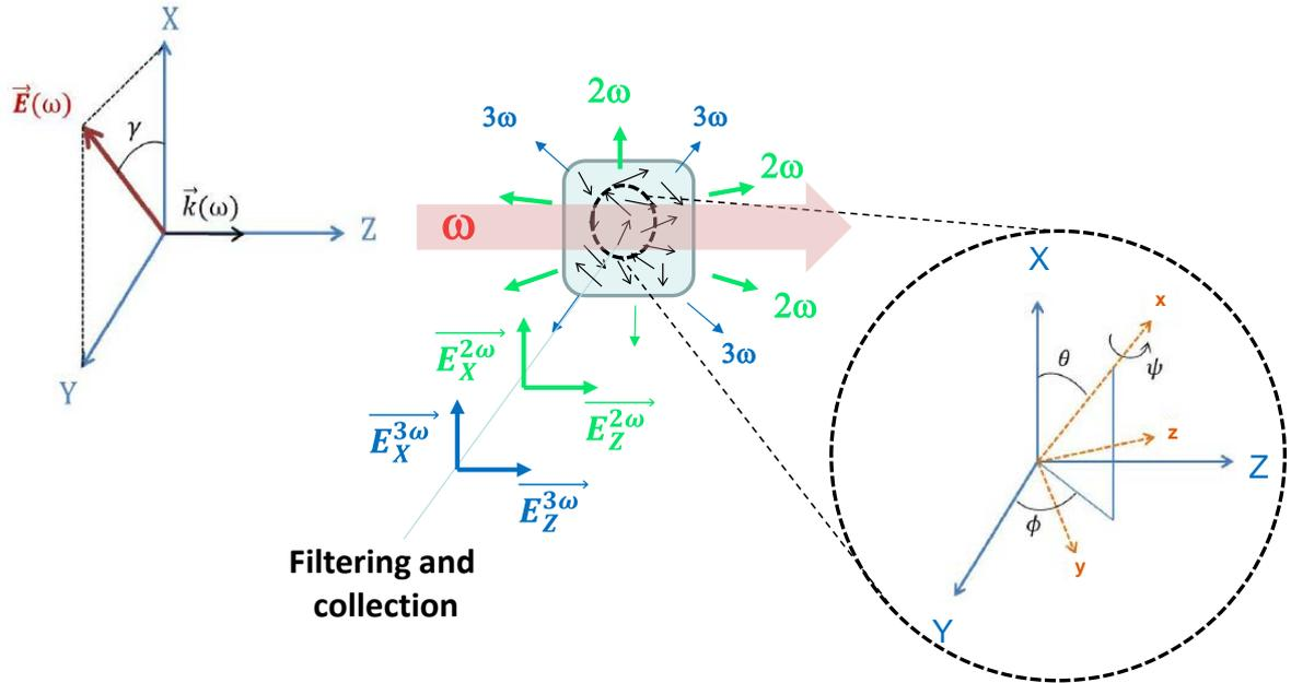
**Figure 3.** Experimental configuration for SHS and THS measurements with an incident linear polarization in the (X,Y) plane and a detection along the Y-axis direction. Definition of the Euler angles  $\Omega(\phi, \theta, \psi)$  in the XYX convention leading to the orientation-averaged entities in the (macroscopic) laboratory frame  $\{X, Y, Z\} = \{I, J, K\}$  from the susceptibility tensors expressed in the (microscopic) crystal frame  $\{x, y, z\} = \{i, j, k\}$
