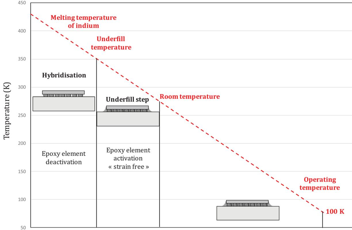
Fig. 8. Thermal loadings considered in the model.
