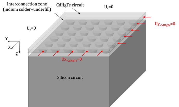
Fig. 7. Boundaries conditions considered for the 3D model.
