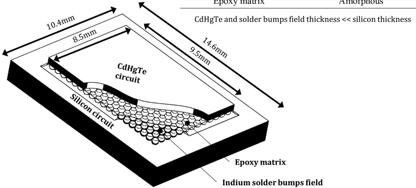
Fig. 1. Architecture of the IR detector considered.
