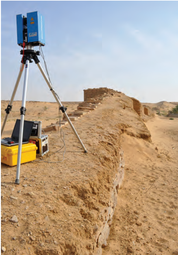
Fig. 4. Shot n. 0. The device has been placed on the wall to assure the links of the two shot lines of the walls
