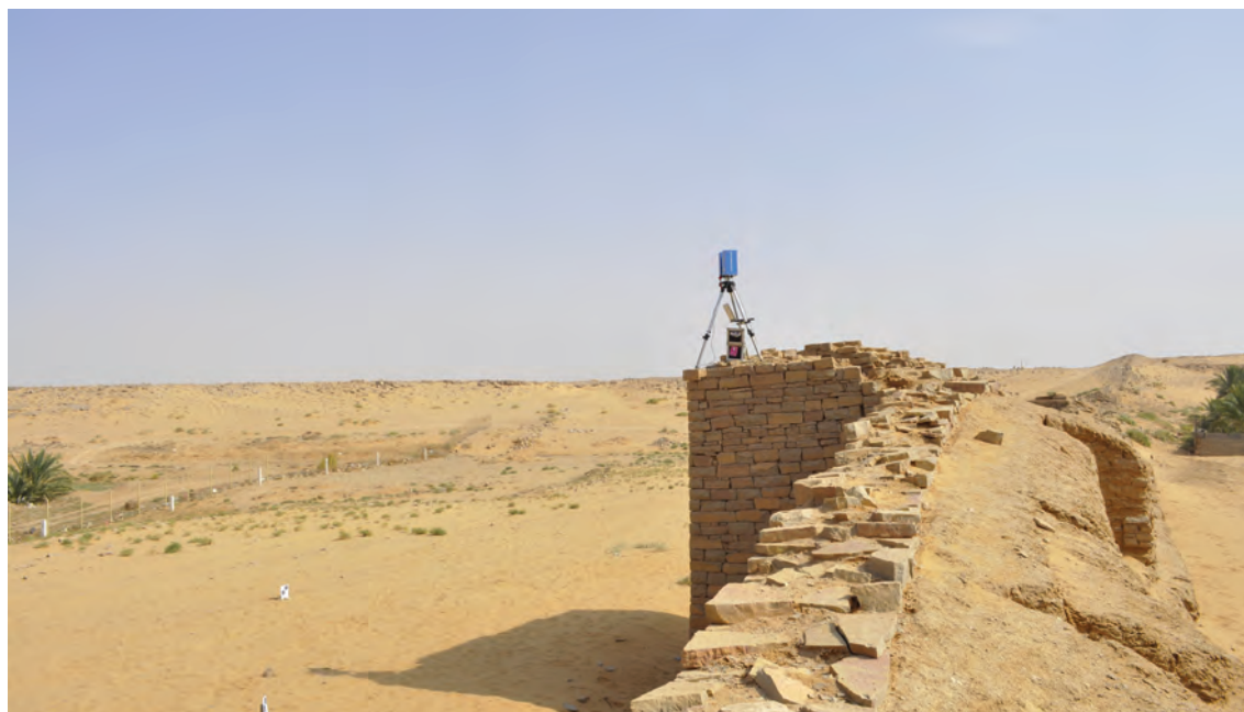
Fig. 9. The laser scanner was placed on the top of the tower to acquire the internal part of the stronghold
