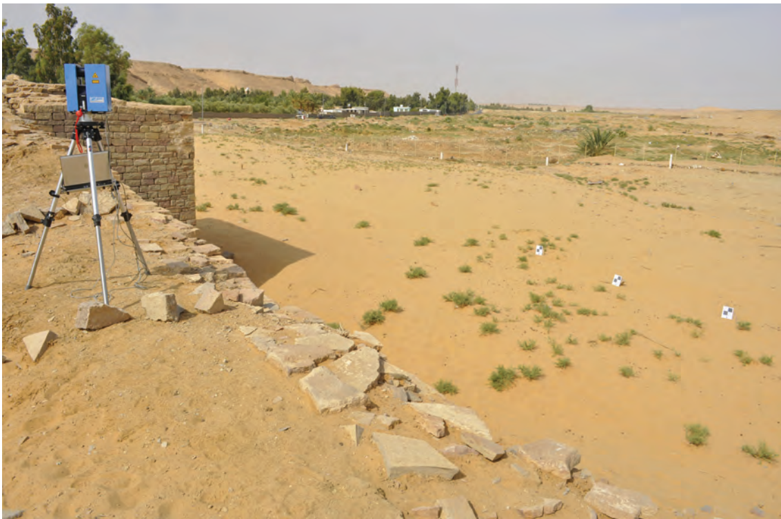
Fig. 7. Shot n. 11. The point-cloud registers the flat targets placed on the outer part of the walls
