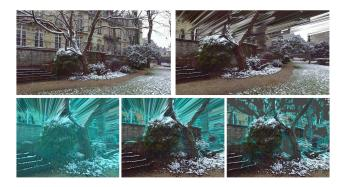
Figure 6: Meshes created from the 360° color image and depth map of the Snow [6] dataset. Top: the added geometry provides motion parallax, but creates stretching artifacts when moving away from the initial viewpoint. Bottom: our toolkit can create depth-based meshes with smaller triangle counts (middle) than full pixel meshing (left), and remove stretched triangles at disocclusion boundaries (right).
