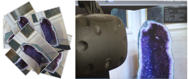
Figure 1: From unstructured sets of photographs to interactive VR scenes providing motion parallax and view-dependent highlights. We present an open toolkit we developed to help casual content creators render real-world scenes in virtual reality.
