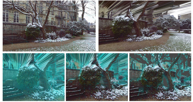
Figure 6: Meshes created from the 360° color image and depth map of the Snow [6] dataset. Top: the added geometry provides motion parallax, but creates stretching artifacts when moving away from the initial viewpoint. Bottom: our toolkit can create depth-based meshes with smaller triangle counts (middle) than full pixel meshing (left), and remove stretched triangles at disocclusion boundaries (right).
