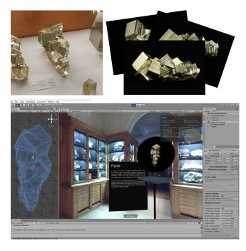
Figure 2: Using COLIBRI VR to render minerals as interactive assets in a VR museum. Top: a pyrite in its museum stand, and photographs of the pyrite used as input for the process. Bottom: the rendered 3D mineral and the toolkit's interface in the Unity game engine.
