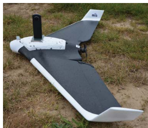
Figure 6. Aerial robot: The twin-fisheye camera was mounted on the Disco using a custom-made expanded polystyrene hull.
