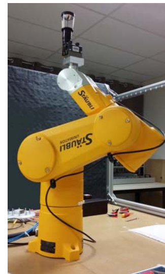
Figure 4. Industrial robot: Stäubli TX60 inside its cell.
