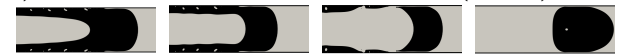
FIG. 1: Transition from a liquid plug to a long levitation drop. a) Scheme of the experimental device. (b) Snapshot of an experiment: a 100 cST silicone oil liquid plug of length 19 mm is pushed inside a capillary tube of radius R = 0.5 mm by a constant flow of air ( Q = 11 mL/min) with a syringe pump, leading to a velocity of the rear interface U of 0.6 ms -1 (corresponding to a capillary number Ca_a^l = \frac{\mu_l U}{\sigma} = 2.8 , with \mu_l the liquid dynamic viscosity and \sigma the surface tension). Image 0 shows the initial plug shape before actuation. Image 1 ( t = 0 ms) shows the deformed rear interface and the inverted front interface when the plug is pushed by a flow of air. Image 2 ( t = 0.6 ms) shows the evolution of the liquid plug and the appearance of a thin film of air surrounding the liquid at the front of the plug. Image 3 shows ( t = 2.3 ms) the drop detachment and Image 4 shows the detached long liquid drop stably propagating in the tube. (c) Numerical simulation of the previous experiment with the same flow parameters: black is silicone oil, white is air.
