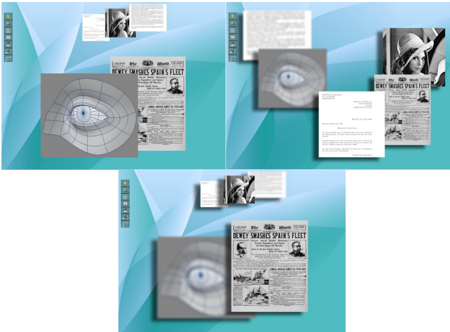
Fig. 4. The upper left desktop is visualized with “relevance” semantic value as scale visual factor. The upper right picture is displayed with blur effect as completion factor. The lower picture is an example of semantic composition of the two previous semantic values.
