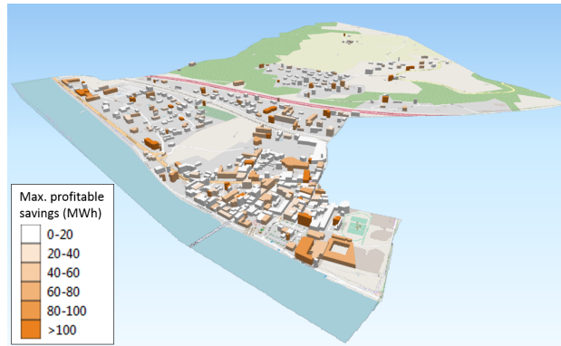
Figure 6: Visualization of maximum profitable savings on a map to enhance decision-aiding. Map background from OSM [52].
