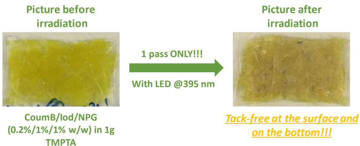
Figure 8. Composite produced upon Near-UV light (LED@395 nm), Belt Speed = 2m/min, using the free radical polymerization (FRP) in the presence of glass fibers/acrylate resin (0.2% CoumB + 1% Iod + 1% NPG in TMPTA). Glass fibers: ~ 2mm of thickness for one layer; 50% glass fibers/50% organic resin.
