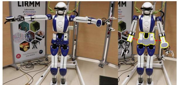
Fig. 4. Initial posture and the pairs of bodies concerned by the collision avoidance constraint (highlighted with yellow contour).
