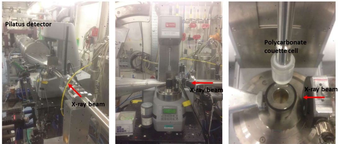
Figure S 1 – Rheo-SAXS apparatus used at the BM29B beamline at ESRF synchrotron (Grenoble, France). A MCR 501 rheometer (Anton Paar, Graz, Austria) equipped with a Couette polycarbonate cell (imposed gap = 1 mm) is employed. A radial configuration is used during the Rheo-SAXS study.
