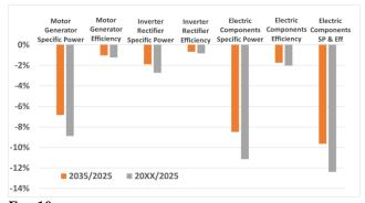
FIG.10: MTOW VARIATIONS VERSUS TECHNOLOGICAL IMPROVEMENT OF THE ELECTRIC CONVERSION CHAIN FROM THE 2025 TARGET
