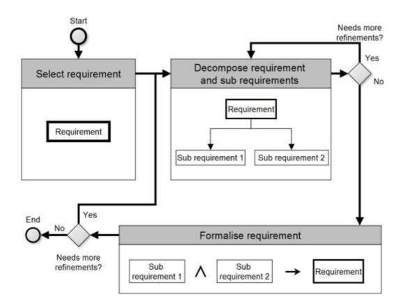
Figure 3. The three main steps of the decomposition and formalisation methodology. Adapted from (Peres et al., 2012)
