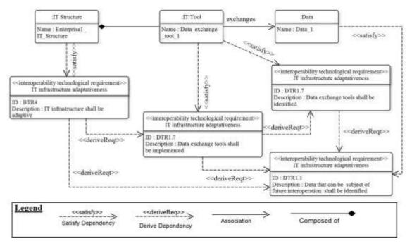
Figure 10. The IRs interdependences based on the U logical connector using SysML notation (OMG, 2017a)
