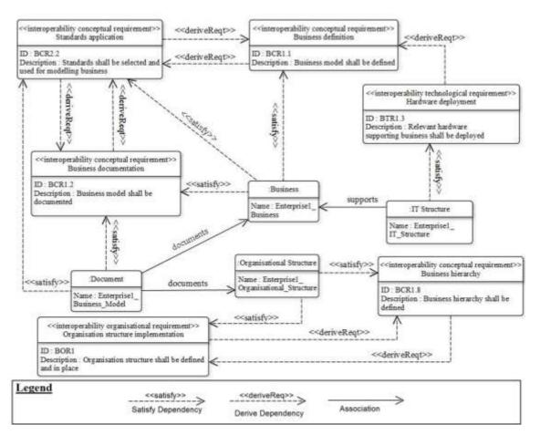
Figure 8. The IRs interdependences using the SysML notation (OMG, 2017a)
