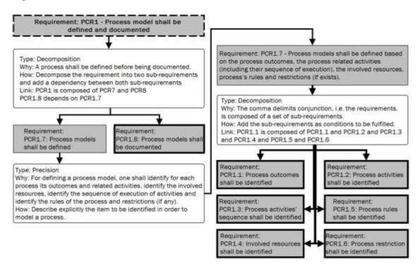
Figure 5. Decomposition of the requirement PCR1
