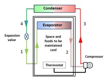
Figure 1 - Schematic representation of a Vapor Compression-Refrigeration cycle.
