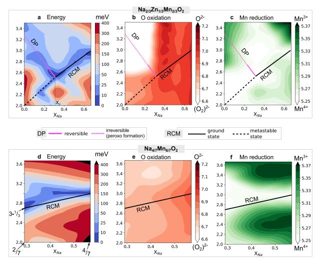
Figure 9: Energy landscapes, Bader populations of most oxidized oxygen and most reduced Mn of  $Na_xZn_{1/3}Mn_{2/3}O_2$  (resp. **a**, **b** & **c**) and  $Na_{4/7}Mn_{6/7}O_2$  (resp. **d**, **e** & **f**) (see fig.8 for details).
