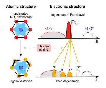
Figure 1: Oxygen oxidation creates a hole in the  $|O_{2p}$  band (top). The Fermi level degeneracy in this localized band is unstable (purple line). Oxygen pairing (distortion) splits the  $|O_{2p}$  band thus lifting the degeneracy and stabilizing the structure (bottom).
