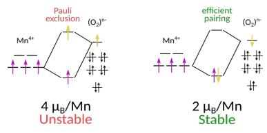
*Figure S9: Effect of Oxygen spin state on the reductive coupling mechanism (RCM).* Parallel Mn and O spin configuration (left) is not stabilized by Mn-O<sub>2</sub> interaction. Antiparallel configuration (right) allows efficient coupling and stabilization. Thus RCM leads to spin decrease, as confirmed by bader charges, see below, fig. 10.
