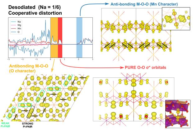
Figure S14: Analysis of the symmetry of empty states in the desodiated  $Na_{1/6}Mg_{1/3}Mn_{2/3}O_2$ : the electronic states lying within the energy range indicated in the pDOS (top left corner) are visualized using a Partial charge density projection (PARCHARG).
