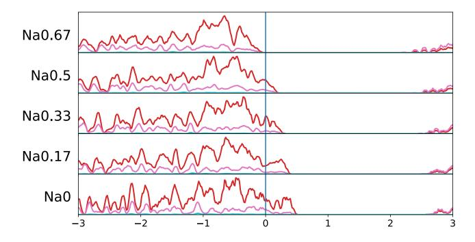
Figure S8: Single point calculation of Density of states (DOS) for  $Na_xMg_{1/3}Mn_{2/3}O_2$  at various x, where the sodium content is given at the right of each DOS. Red curves curve stands for O while pink curves stands for Mn. The Fermi level is highlighted by a blue line.
