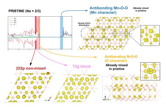
Figure S13: Analysis of the symmetry of electronic states near the band-gap in the pristine  $Na_{2/3}Mg_{1/3}Mn_{2/3}O_2$ : the electronic states lying within the energy range indicated in the pDOS (top left corner) are visualized using a Partial charge density projection (PARCHARG).
