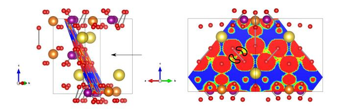
Figure S6: ELF value in a plane passing by the O-O pairs for  $Na_{1/6}Mg_{1/3}Mn_{2/3}O_2$ (cooperative distortion). Interval : 0.4 % (blue) - 0.7% (red) of maximum value. Grey lines in the structures indicate short O-O distances (<2.5A)
