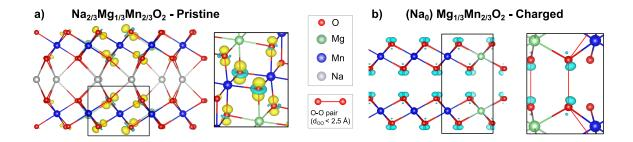
Figure 5: Fukui functions of pristine and charged  $Na_xMg_{1/3}Mn_{2/3}O_2$ . The electronic reorganization upon addition or removal of 1 electron at constant structure causes an increase (blue) or a decrease (yellow) in the electronic density. **a**) Fukui – of the pristine compound (1 electron removed). **b**) Fukui + of the fully charged compound (1 electron added). Both isosurfaces have values of 2.10<sup>-3</sup>. Insets : close-up on oxygen pairs. See Methods section for further details.
