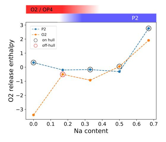
Figure S7: Enthalpy of O2 release reaction during anionic redox and phase stability. A negative enthalpy indicates a favorable release reaction, a positive value indicates a stability. A second order phase transition occurs between x=0.3 and x=0.1 Even though anionic redox destabilizes both stacking phases, the O2 phase is more prone to oxygen release than P2 phases, especially is we discard the off-hull point, added here for completeness.
