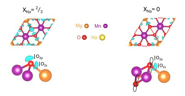
Figure S4: Molecular orbital description of oxygen geometry in  $Na_xMg_{1/3}Mn_{2/3}O_2$  Crystal structure with zoom on oxygen, with E.L.F. isosurface locating non bonding doublets and insight from Lewis structure. Left : for  $x_{Na}=2/3$  Right :  $x_{Na}=0$ .
