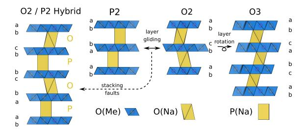
Figure S1: Stacking phases in Na-deficient compounds as classified by Delmas & al.<sup>3</sup>
