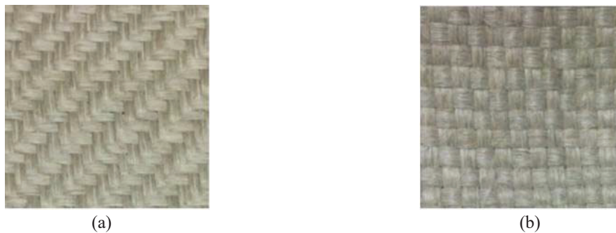
FIGURE 4. Textiles used – (a) Sized up linen, Serge 2x2, (b) desized linen, plain weave (B)
