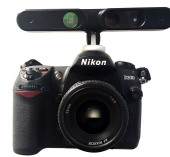
Fig. 10. Experimental platform with Xtion PRO sensor coupled to a DSLR Nikon camera.
