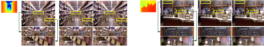
Fig. 5. Examples of synthetic defocused images generated from an image of the NYUv2 database for two camera in-focus plane settings: 2 and 8 m.
