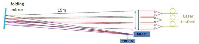
Figure 5. Schematics of the experimental setup for 30-m range TIL-CBC with optical path folding mirror to double the range of the experiment. The interference pattern is monitored with a camera located at the same distance from the laser as the target.
