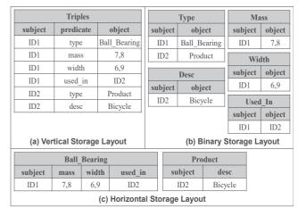
Fig. 5 Example of the used storage layouts
