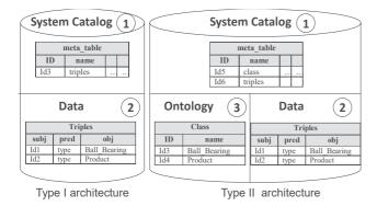
Fig. 6 Type I and type II architectures of OBDBs
