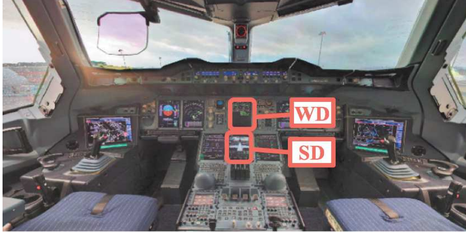
Fig. 5. Warning and system displays in A380 cockpit.
