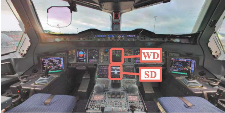
Fig. 5. Warning and system displays in A380 cockpit.
